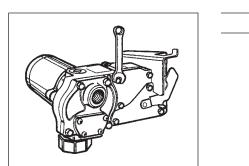
• Remove the torx head screw, then remove the switch assembly. (Figure 13)
