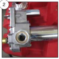
Pump has a free swivelling nut that will attach to the captured nut provided
